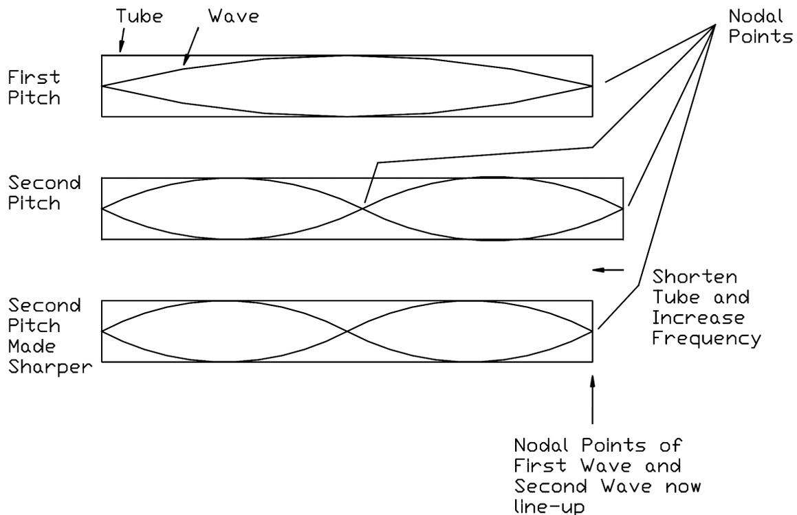
Figure 32. Aligning nodal points on a chanter
